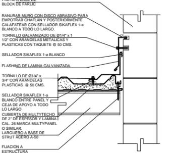
05 DETALLE DE PRETIL CON FLASHING
