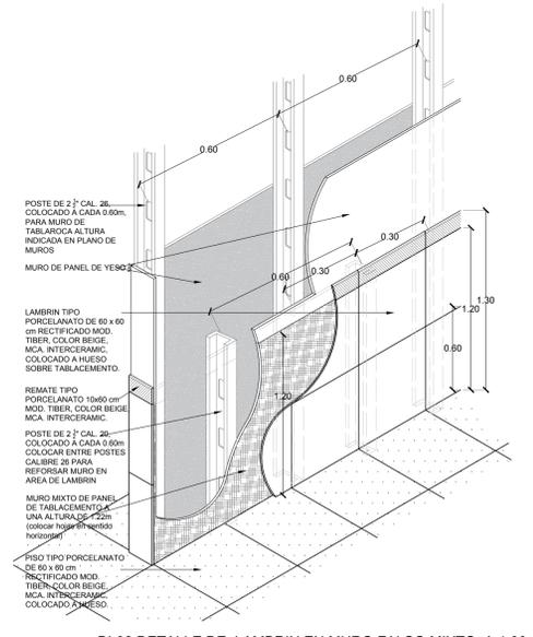
**D-02 DETALLE DE LAMBRIN EN MURO FALSO MIXTO A 1.30m**
