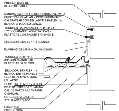
**05 DETALLE DE PRETIL CON FLASHING**
